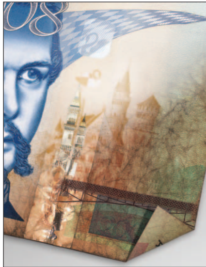
A G&D house note after having undergone the Life Time Test cycle
